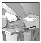
**C.** Set a jigsaw to 45 and use it to cut between the lines.
