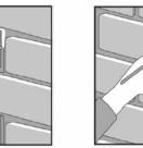
**5.** Once the whole wall has been covered with the panels fill the joints and screw wholes with glue- paste.
