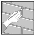
**6.** When filled remove any irregularities in the paste with a fine brush. Once the paste is completely dry (approx. 24 hours), paint the joints and screw holes with ENVIROCLAD special paint, to give a perfect finish.
