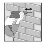
**3.** Fit the panel to the wall and drill through the panel directly into the wall using a 6mm drill bit. Put the screw into the wall-plug and introduce both into the hole in the panel. Push and screw them in until the panel is securely fixed. (e.g. "Fischer" 6mm wall plug and 4.5 x 40 screws are recommended). Use as many screws per panel as needed.
