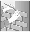
**A.** When you reach an external corner, mark on the inside of the panel line a line where the panel meets the wall. (This will be the inside line of the cut)
