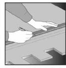
**A.** From this line, mark all parallel line away from the wall at a distance equal to double the thickness of the panel - between 2 and 4 cm depending on the model. (This will be the outside line of the cut)
