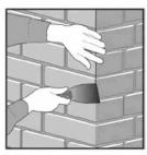
**D.** Offer the panel upp to the corner and fix it to the wall Fill the joint and the holes.
