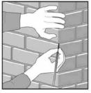
**E.** When the joint is filled, remove any irregulatities in the paste with a fine brush.
